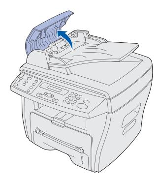
2 If more than one inch of your document has passed beneath the ADF roller, close the ADF top cover, and then proceed with the instructions for clearing a jam in "Roller misfeed" on page 72.
